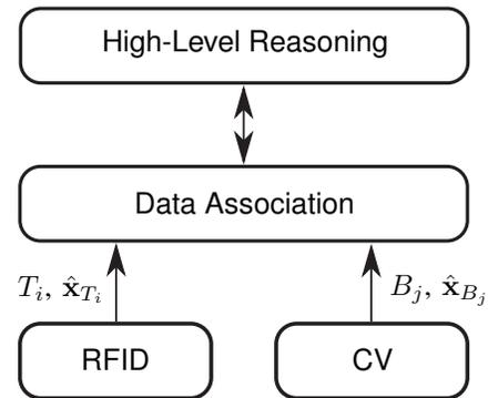
Fig. 1. Block diagram for a combined RFID and CV localization system. The RFID and CV subsystems detect and localize tags  $T_i$  and motion blobs  $B_j$ , respectively. The data association layer subsequently finds the most probable match between identified tags and detected blobs in the scene. Based on the combined information, a high-level reasoning scheme can be employed to provide abstract information rather than low-level trajectory data.
