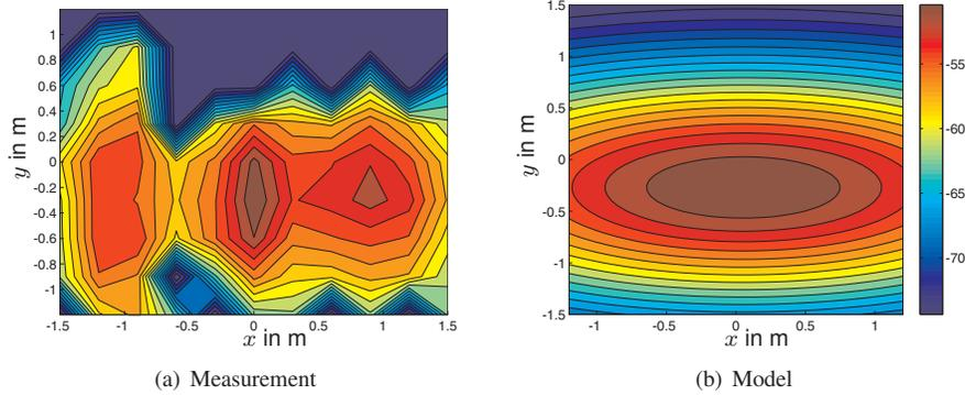
Fig. 9. RFID sensor model: Contour plot. (a) shows the measured interrogation zone (RSSI values) for a  $\Delta x = \Delta y = 30$  cm tag grid and (b) shows the approximation by means of a 2D Gaussian. The considered system comprises a Kathrein Widerange antenna with  $70^\circ / 30^\circ$  half power beamwidth, mounted at a height of  $h = 2.5$  m.
