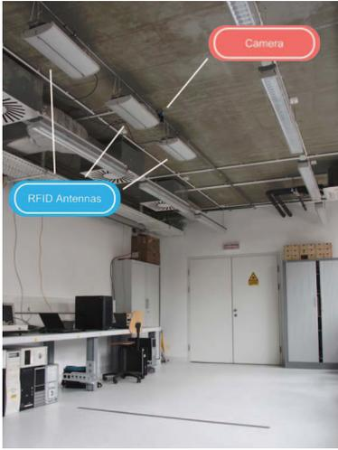
Fig. 3. Setup of the proposed sensor fusion system. The RFID antennas and the camera are mounted at the ceiling to cover a specific region of interest. By means of that, the two sensor modalities can be aligned to operate in a common reference frame.
