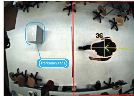
Fig. 5. Motion blob detection and tracking: Camera view of the lab environment shown in Fig. 3. In this scenario, a moving person is identified as blob with ID 36. On the left hand side, there are two stationary tags in the scene.
