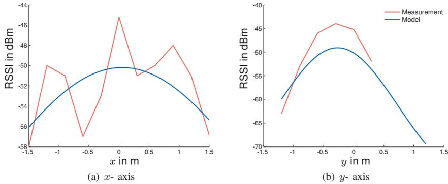
Fig. 10. RFID sensor model for a single antenna: RSSI values along the principal antenna axis for the  $x$ -direction in (a) and the  $y$ -direction in (b), together with the Gaussian approximation. Along the  $x$ -axis, the interrogation zone shows a characteristic peak and two local maxima from the side lobes of the antenna radiation pattern.
