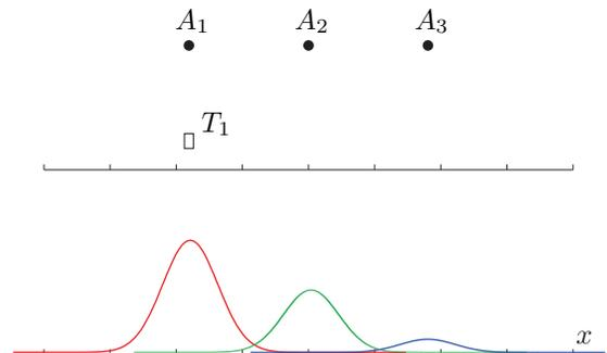
Fig. 2. RFID sensor model for a simplified 1D case with  $K = 3$  antennas. The sensor model incorporates a mixture of Gaussians (MoG) to provide a likelihood for the location of tag  $T_1$  based on the mean RSSI values. The parameters of the mixture model depend on the antenna characteristics (position and radiation pattern) and need to be learned in a calibration step.
