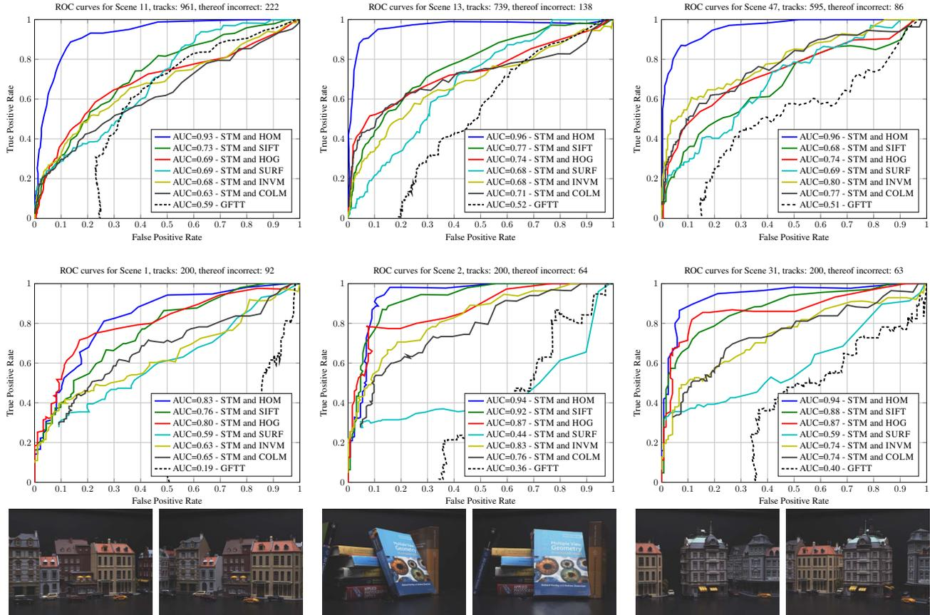
Figure 4. Results for six sample scenes, providing detailed comparison of STM using different spatial feature descriptors with GFTT. The first row shows results for those three scenes that generated the largest number of SIFT tracks (fulfilling Lowe’s ratio criterion over all frames). The second and third rows show three selected results for LK-tracks and the corresponding scenes.
